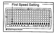
program speed and incline settings for the first period, simply adjust the speed and incline of the treadmill as desired with the SPEED and INCLINE buttons. Every few times one of the SPEED buttons is pressed, one additional indicator will light or darken in the flashing column of the LED matrix.
